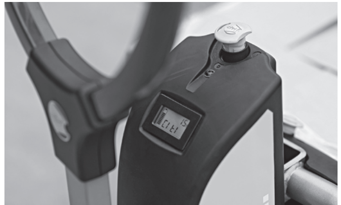
Everything in view, all the time: multifunctional display shows operating hours, warnings, charging status and, optionally, weight
