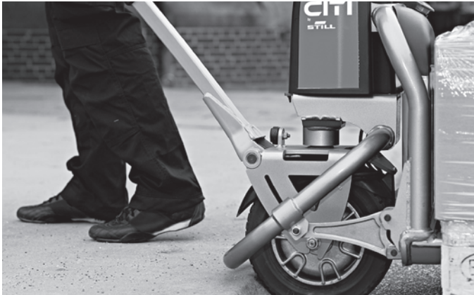
Can be used on any flooring thanks to profiled solid rubber drive wheel
