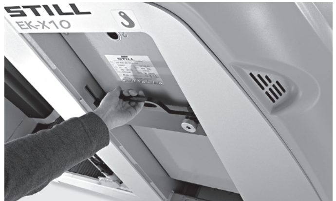
Simple lateral battery change optionally available, and electronic monitoring of battery locking for more operator safety
