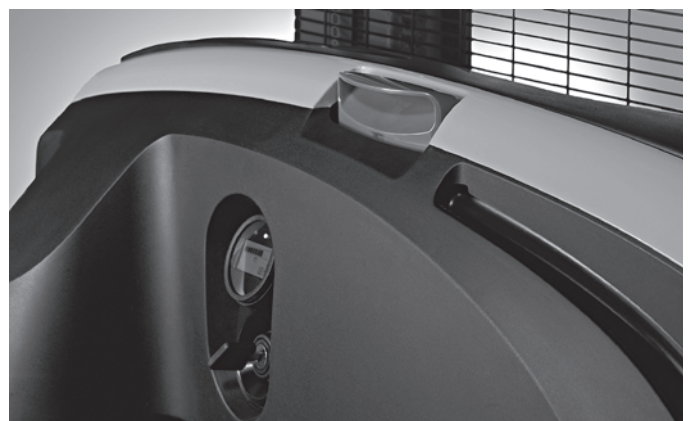
Unauthorised access not possible: access authorisation by key, PIN code, chip or card
